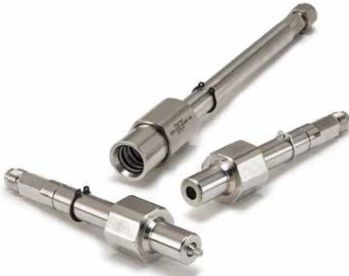
DSH Series couplings are used on subsea and topside RBQ/J - Plates. Typically found in hydraulic pilot applications they replace legacy couplings, pipe nipples, and fittings eliminating potential leak paths and reducing assembly time. The superior valve design of the DSH Series accommodates plate flex up to 0.100 in/2.54mm.
